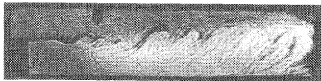
a) Velocity 9.1 m/s, N_{Re} = 5900 \text{ cm}^{-1} , \phi = 0.60 .
