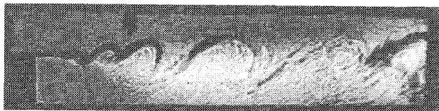
b) Velocity 13.3 m/s, N_{Re} = 8600 \text{ cm}^{-1} , \phi = 0.60 .
